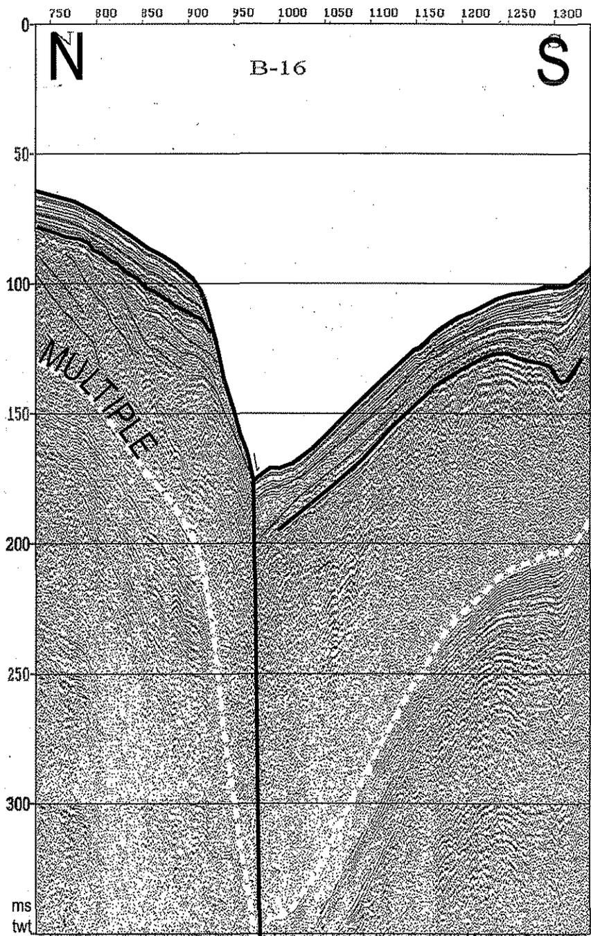
Figure 2 b. Interpreted line drawing of sparker profile B16 showing the the seismic layers and fault ruptures on the sea floor.
