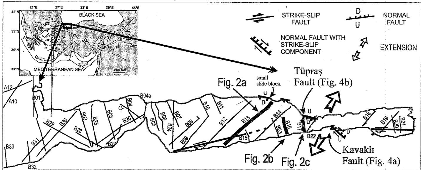
Figure 3. The fault ruptures on sea floor and/or on very near subsurface sediments. This map also shows the shallow seismic profiling tracks utilised in the text and shown in Figure 2.
