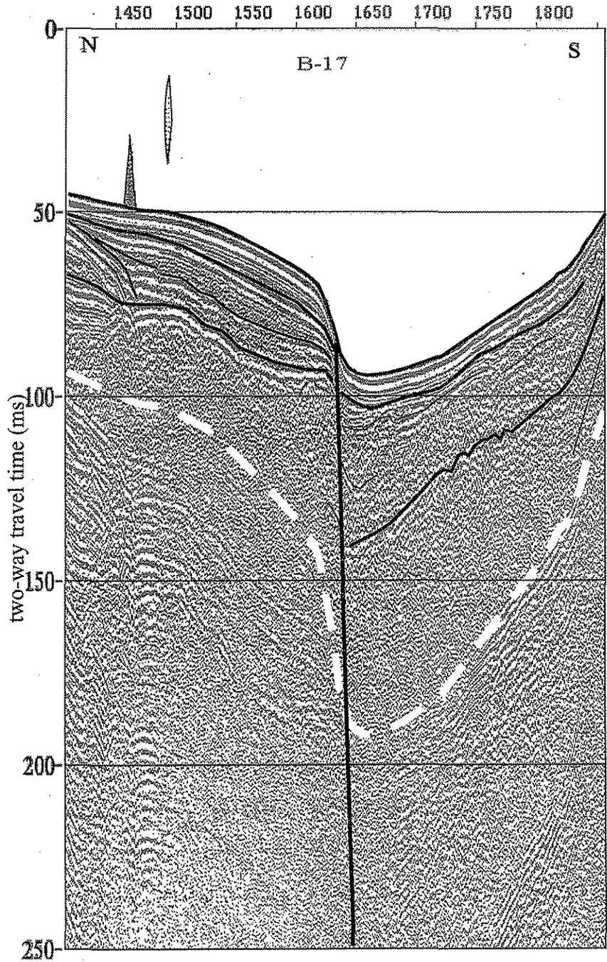
Figure 2 c. Interpreted line drawing of sparker profile B17 showing the seismic layers and fault ruptures on the sea floor. Dashed line stands for multiple. Gas sepages are evident.
