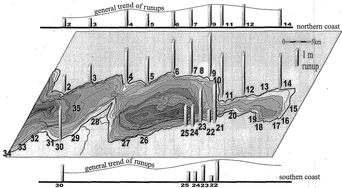
Figure 1. The tsunami runups superimposed on the bathymetry map of the Izmit Bay. See Table 1 for locations.
