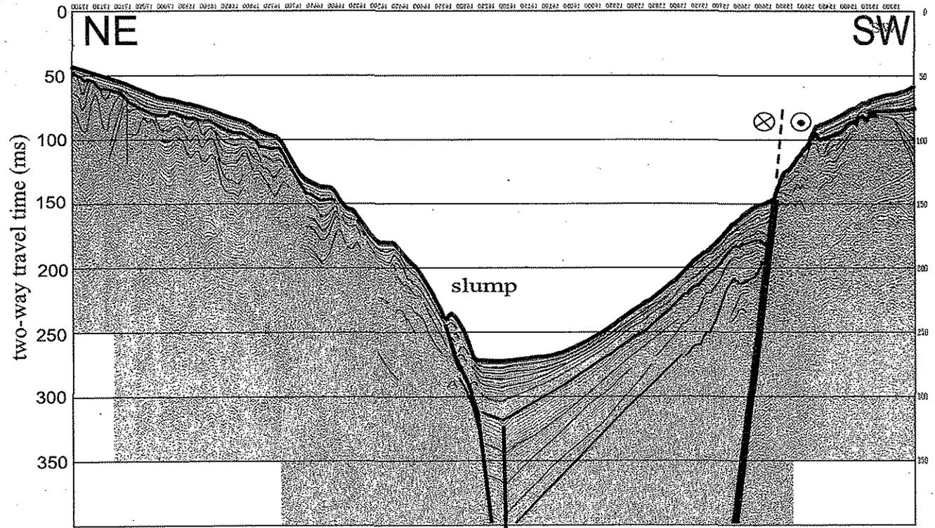
Figure 2 a. Interpreted line drawing of sparker profile B13 showing the layers, slump and faults.
