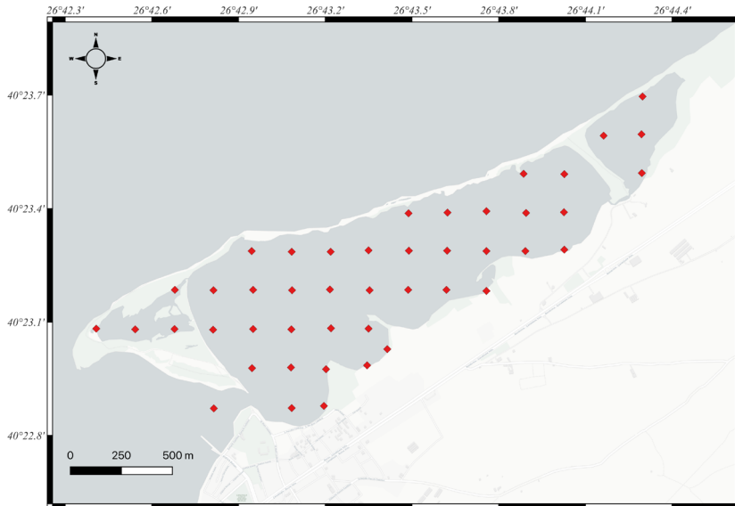
Figure 3. Cartographic representation of the systematic sampling design employed within Çardak Lagoon. The red squares illustrate the 200 \times 200 m spatial grid nodes, delineating the locations targeted for bathymetric profiling and benthic habitat characterisation.
