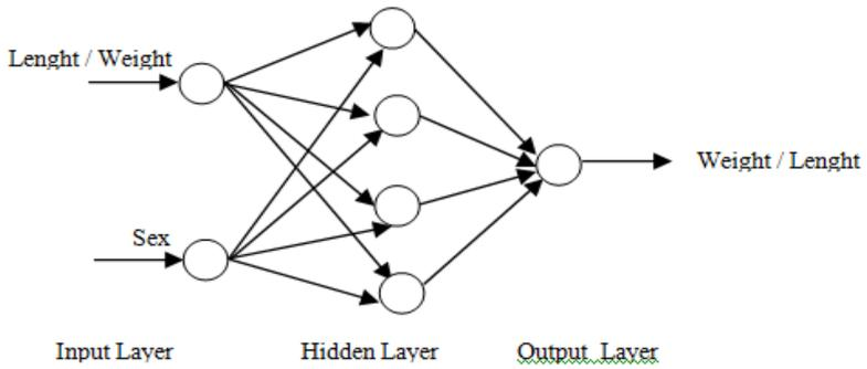
**Figure 3.** The ANN consisted of an input layer with 2 nodes, hidden layer, and an output layer with 1 node to be predicted for crayfish
